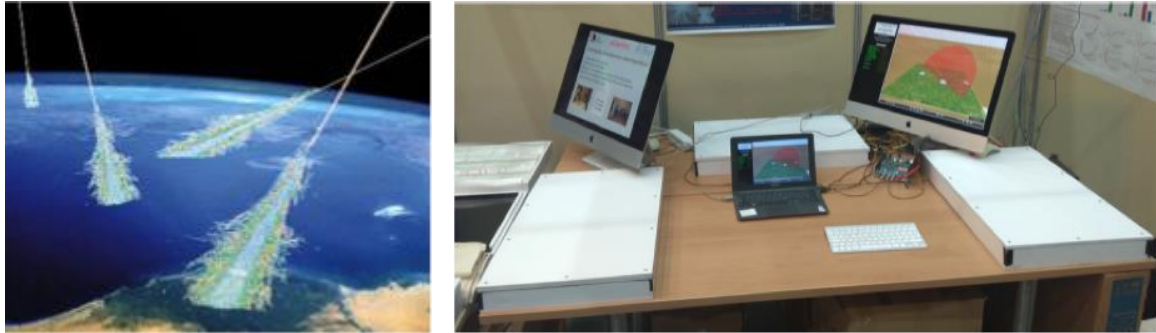
Figure 1. Left: An artistic view of extensive air showers produced in the atmosphere. Right: The \mu Cosmics detection station. The detection units (white boxes) along with the data acquisition board and the station computer (laptop).
